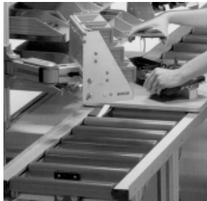
Fig. 1a: Simple roller conveyor for movement of heavy parts.
