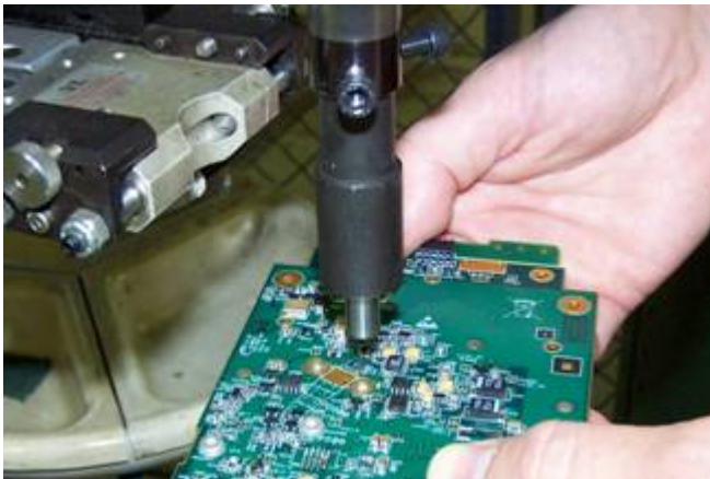
Figure 4: Example of a populated board getting broach fasteners installed at a press. Note the proximity of componentry to the fastener.
