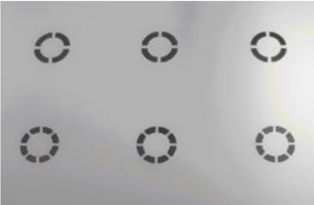
Figure 7: Stencil designs showing spokes to cover the pilot hole in a PC board.
