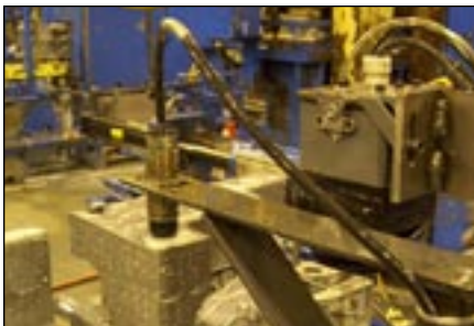
RFID sensor correctly reads build information from electronic tag through pool of cutting fluid.
