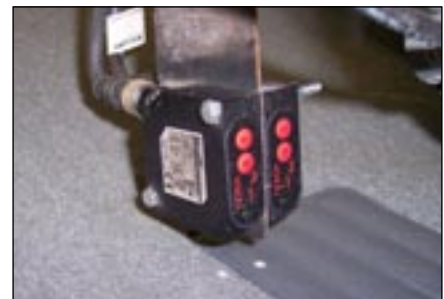
Working together, these two color sensors can exactly match and error proof color of two dissimilar floor mat materials.
