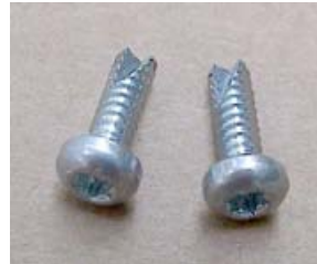
Torx Screw (a 2 nd feed system is tooled for a different screw and allows an automatic tooling changeover)
