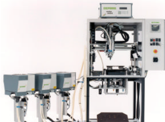
View of complete Screwdriving Unit with the Feeders for 3 different screws
