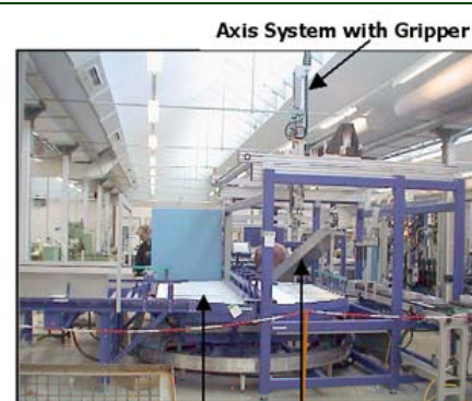
Axis System with Gripper Conveyor with rotary index table Chute for "Bad" parts
