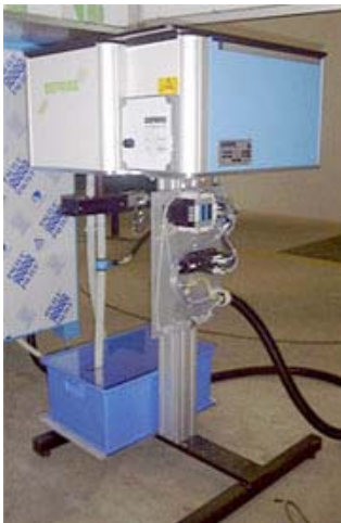
2.5-liter capacity Screwfeeder with sorting device
