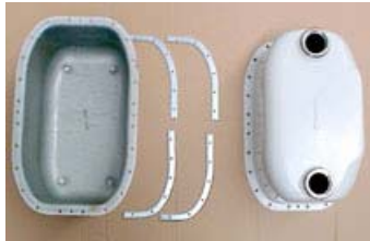
Gas-Meter prior to Assembly
