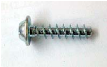
Screw No. 1 is assembled into the pressure sensor at a torque of 2 Nm [17.8 in.lbs.]
