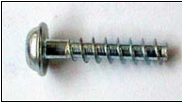
Screw No. 2 is assembled into the suction connector at a torque of 4.8 Nm [42.5 in.lbs.]
