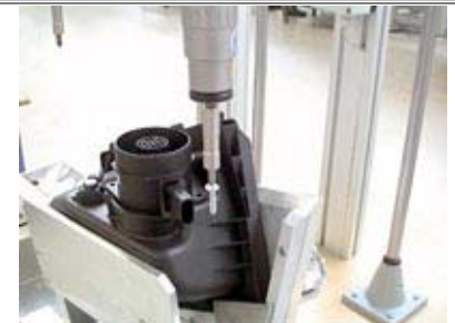
Screwdriver tip showing the magnetic bit with screw
