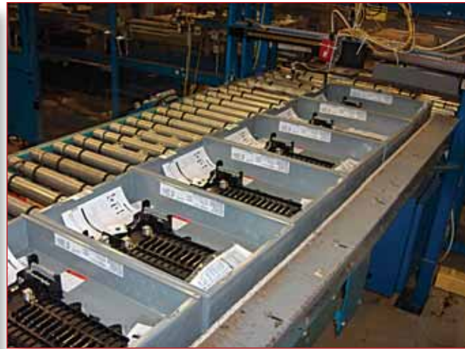
A batch of fully assembled load centers are queued on the packaging line. Covers are packaged separately. Photo by Austin Weber
