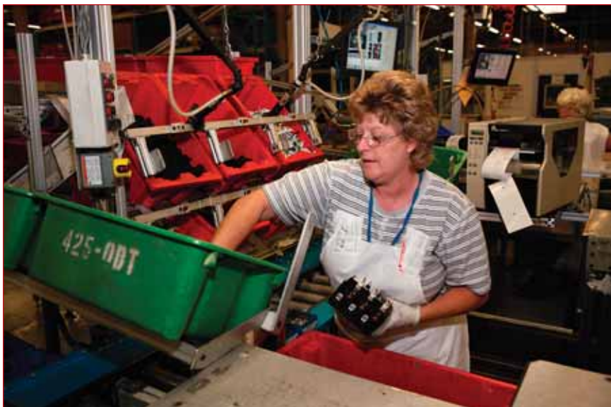
Smart bins are used to error-proof assembly and confirm that each component is correctly picked according to bills of material. Photo courtesy Schneider Electric/Square D
