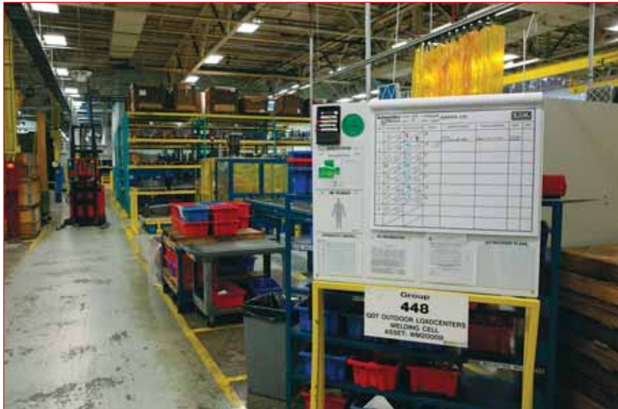
As part of its lean manufacturing initiative, the plant uses group-level short interval management boards. Photo courtesy Schneider Electric/Square D
