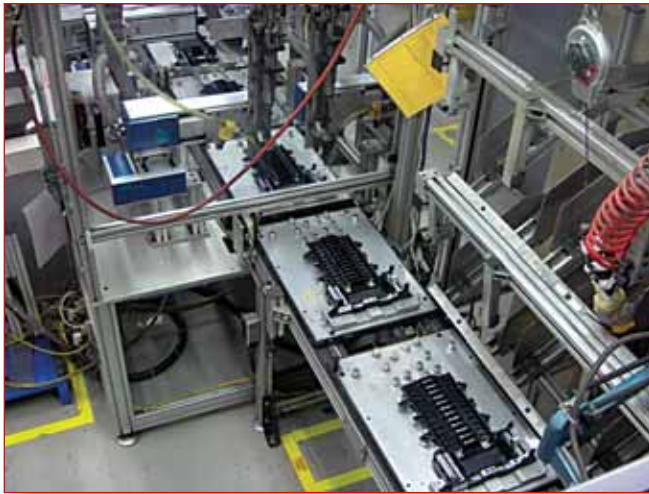
Fully automated pneumatic drivers remove the risk of carpal tunnel syndrome and other injuries that may accumulate over time. Photo by Austin Weber
