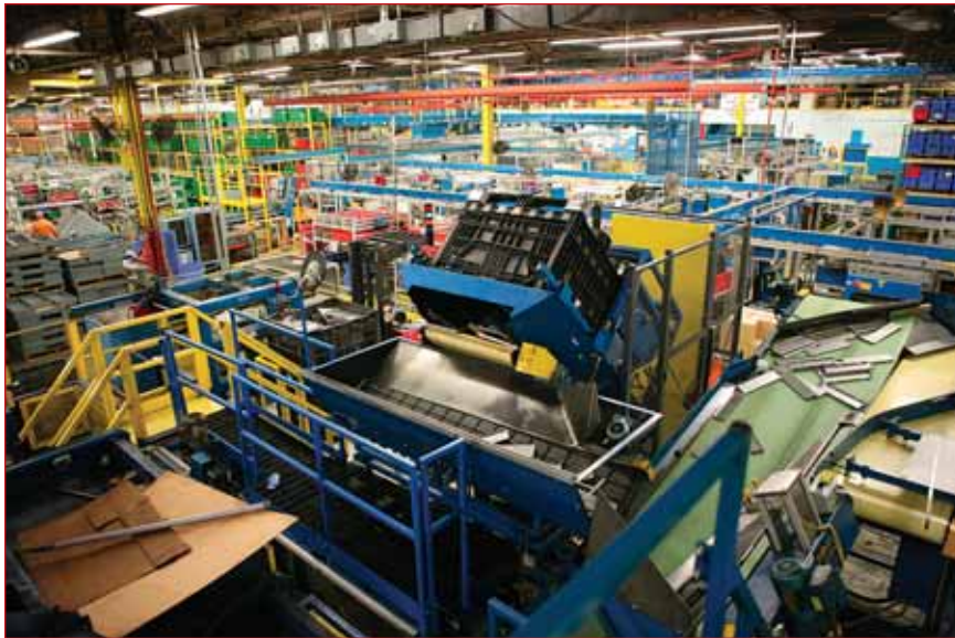
Over the last seven years, the plant has focused on consolidating many manually operated stations into larger, faster automated systems. This new machine center improves welding throughput. Photo courtesy Schneider Electric/Square D
