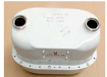
Gas-Meter after Assembly
