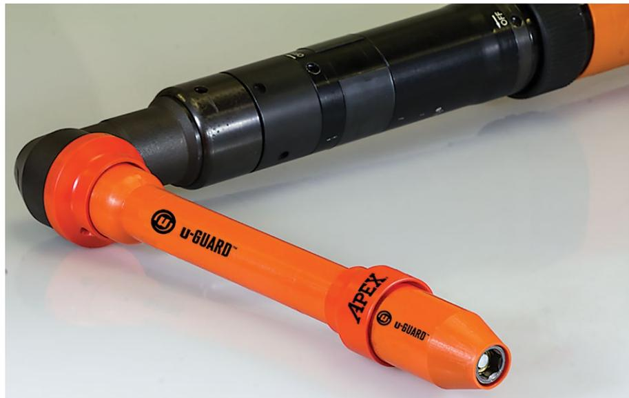
**APEX u-GUARD UGS Series bits, bit holders, sockets and extensions are surrounded by a soft plastic cover. The drive tool can spin freely inside the cover, preventing contact between the tool and an assembler's fingers.**
