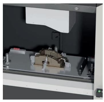
Simultaneous welding, combined with the Branson GLX servo lift table actuation technology results in a high-speed weld cycle that typically ranges from 0.5 to 5 seconds, depending on part material and geometric complexity.
