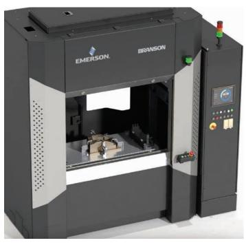
The lift table is positioned low to minimize potential back strain of workers.
