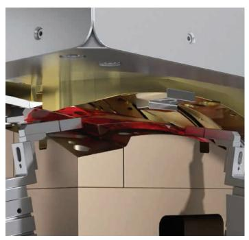
With no movement of the parts during joining, this leads to a more precise weld and hermetic seals can be created if required.
