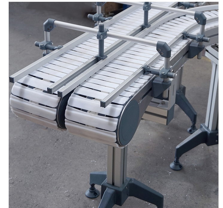
In this example two VersaFlex A17 models share a common support structure before one curves to the right and the other continues straight.
