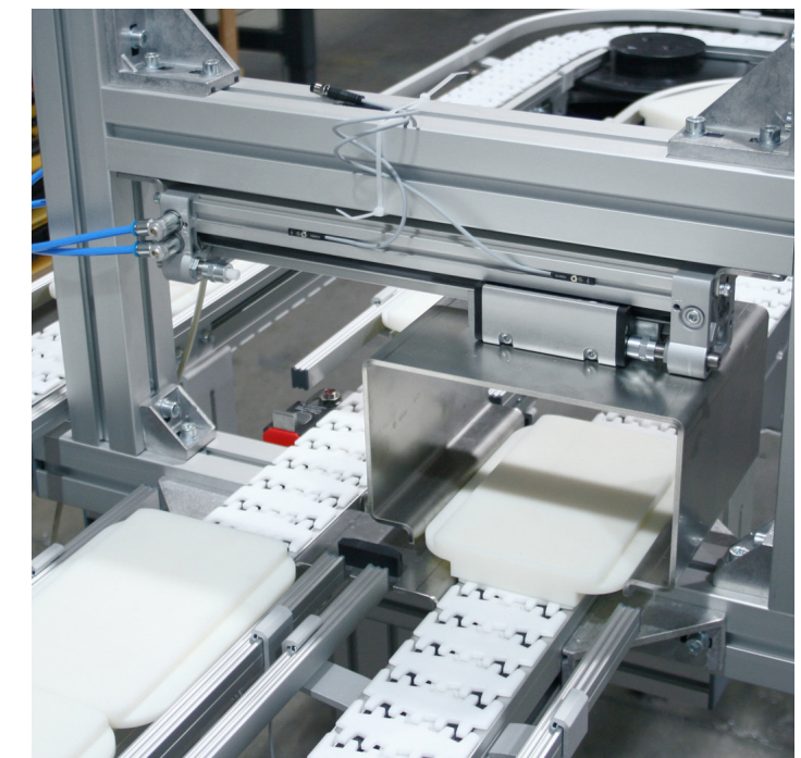
A custom pick and place unit is used to move pallets from one VersaFlex P08 conveyor to another.
