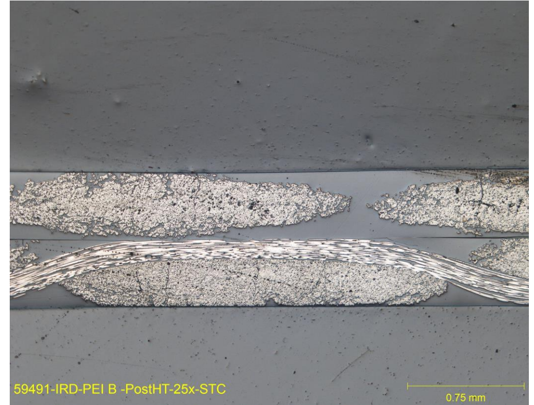
Carbon fiber filled PEI welded to itself
