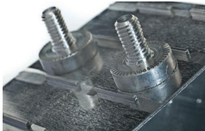
Welding threaded studs to a deep-drawn Al housing (source: Telsonic)
