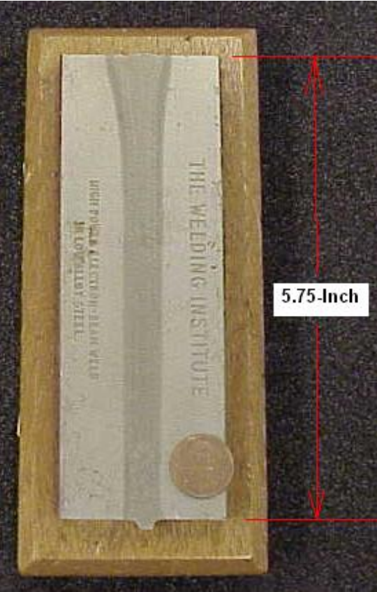
5.75-in.-Deep EB Weld
