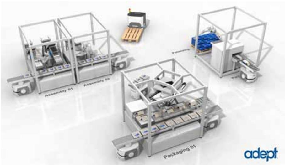
Flexible robotic workcells being fed by Adept Lynx AIV's.
