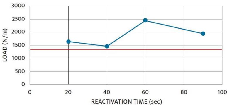
In The manufacturer’s specifications called for the ability to pass a peel test at 1,400 N/m for adhesion of a vinyl skin to a Teflon-coated spacer. In figure 5, the red line indicates this spec. Coat weights were 300 gsm wet. The blue line shows that, at a reactivation temperature of 70 C, 5101 P passed the manufacturer’s strict specification at 20, 40, 60 and 90 seconds, consistently meeting requirements
