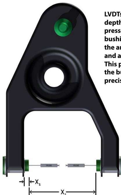
**LVDTs are used to measure the depth of bushings as they are pressed into a control arm. The bushing is pressed in partway, the arm is allowed to relax, and a measurement is taken. This process is repeated until the bushing has been located precisely.**
