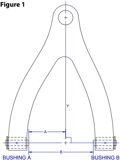
An engineering drawing of a control arm assembly lists dozens of dimensions, but only two really matter. (See Fig. 1.) One is the distance between the bushings (Line B). That dimension has to be held, because when the control arm is installed, it slides over another part and gets secured with pins. If that dimension is too tight, the arm won't fit. If it's too loose, the assembly will be sloppy.
