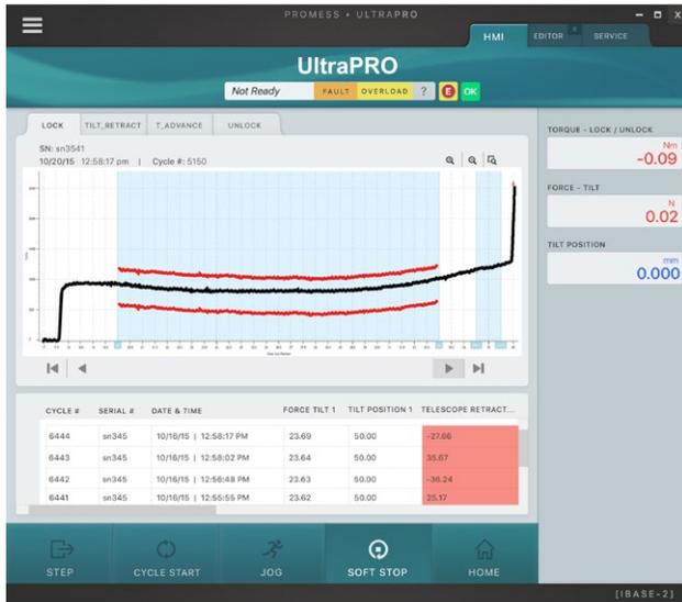
Measuring both force and distance during the pressing operation can give assemblers valuable information about the quality of the parts and the assembly.
