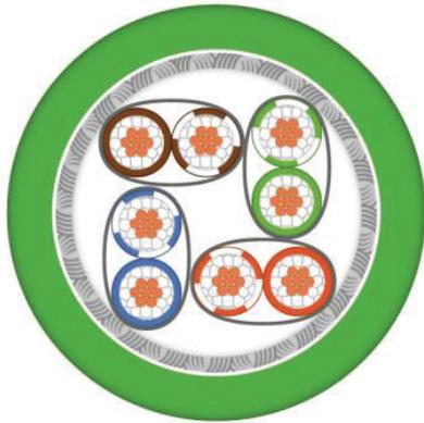
*ETHERLINE® Ethernet Cat.7 cable's robust PUR outer jacket is highly resistant to mineral oils and abrasion, and its double-shielding ensures transmission reliability.*
