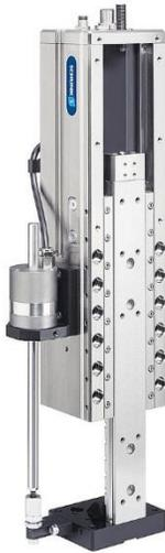
The smart 24 V SCHUNK ELP linear axis is now also available with an electrically activated holding brake.
