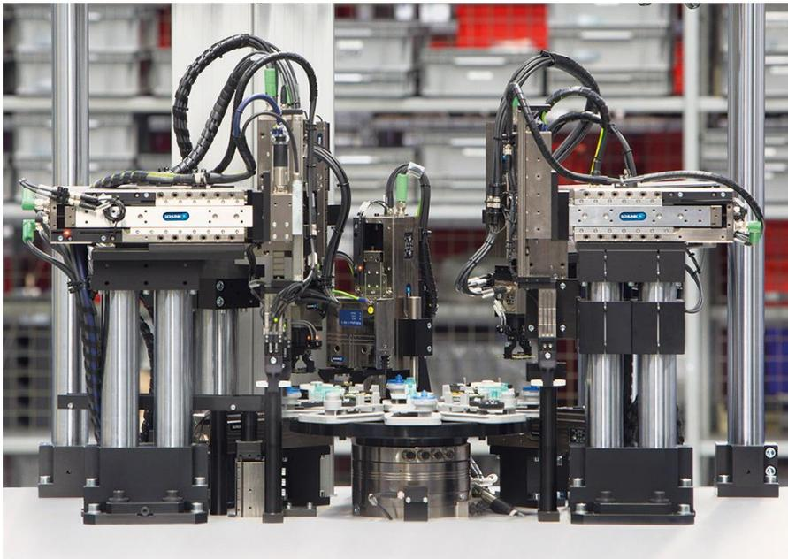
SCHUNK ELP linear axes, SCHUNK EGS rotary gripping modules, and SCHUNK EGP grippers can be combined with efficient 24 V assembly systems. Customers benefit from 24 V technology with minimum commissioning and low maintenance costs, high energy efficiency, and low life cycle costs.
