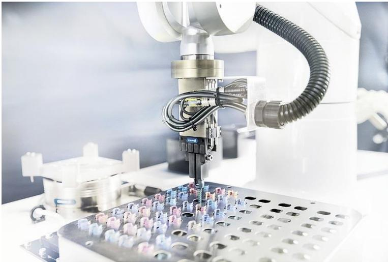
The 24 V SCHUNK EGP gripper for small components is specially designed for assembly applications.
