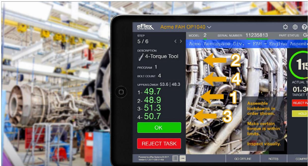
JEM does not directly control these devices. Rather, it tells them what program to run based on whatever model or variant is being produced. It waits for the hardware to complete the task, and receives any data—an image, a gauge measurement, a torque value, etc.—the hardware might collect.
