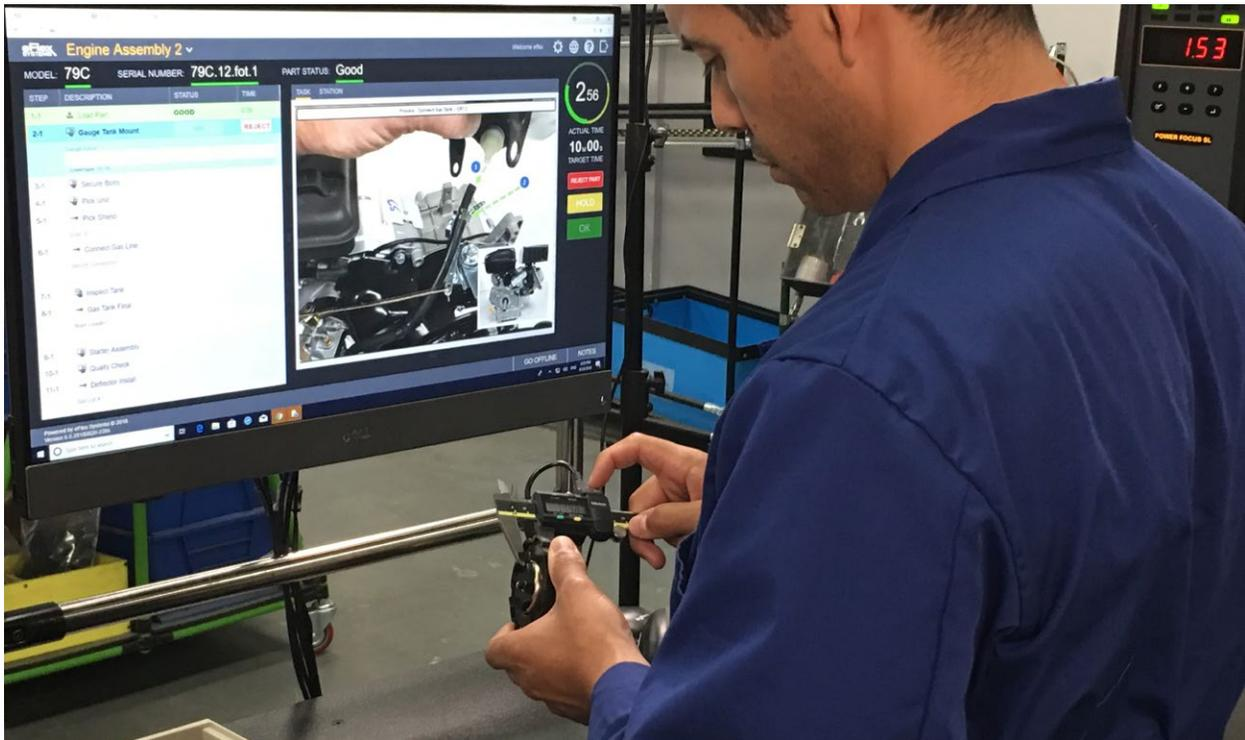
With JEM software, every task has fields that can be configured to capture data. So, for example, as assemblers cycle through a set of instructions, the software can record how long each task took to complete. Such time-study data is invaluable for continuous improvement activities and worker training.
