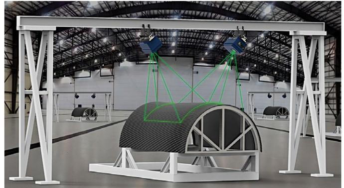
**M**uch of today's manufacturing involves the use of physical templates which can be costly and cumbersome. To increase efficiency and reduce scrap/rework, forward-looking manufacturers have turned toward Laser Projection for templating in applications such as assembly, composites layup, welding, verification, and paint templating.
