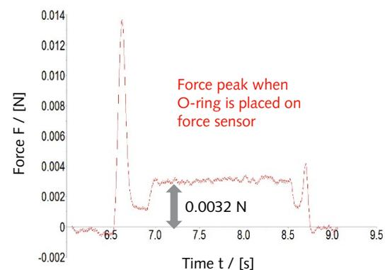
Figure 4: The sensor detects the force impact from the O-ring
