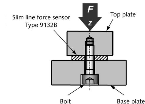
Figure 10: Sensor integrated into a mechanical structure
