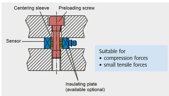
Figure 6: Installation with preloading screw
