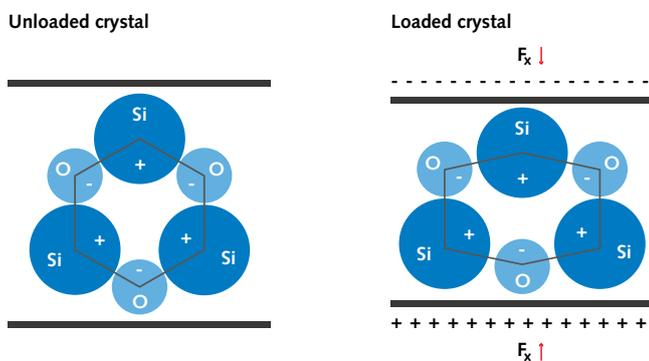
Figure 1: Principle of the longitudinal PE effect
