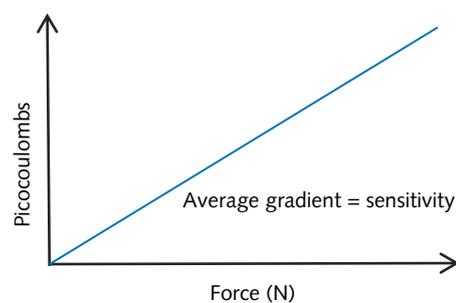
Figure 2: Force versus charge in (pC)
