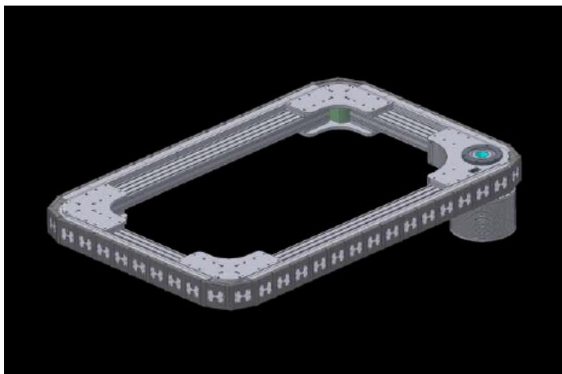
The most noticeable difference is the LATC has a rectangular configuration that provides useable precision stations on all four sides of the conveyor. This offers the customer more stations to work with where highly accurate processes must be performed.
