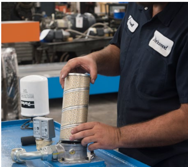
Figure 3: Performing regular filter changes and maintaining oil cleanliness are vital on a fluid power system.
