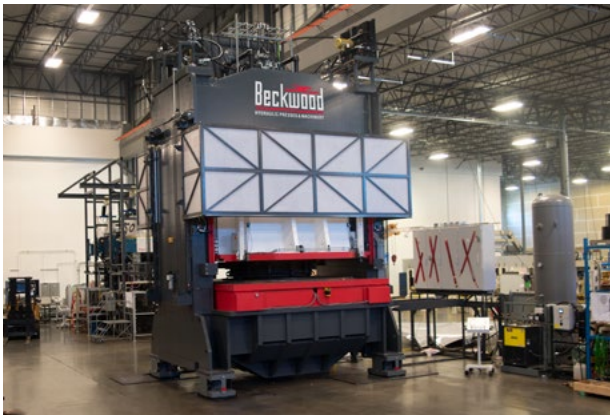
Figure 2: 3,500-ton hydraulic press with hydraulic bed shuttle used to bulge-form stainless steel tankheads.
