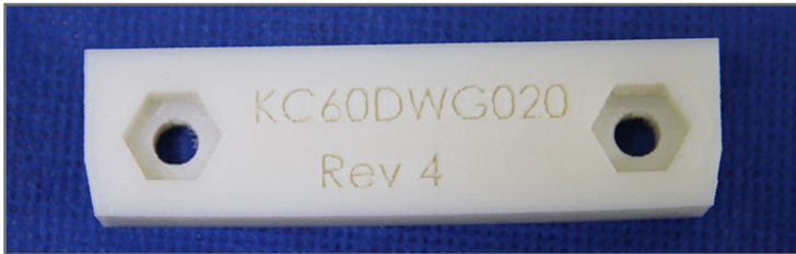
Each part produced on a 3D printer can be uniquely identified with its own rev control number.
